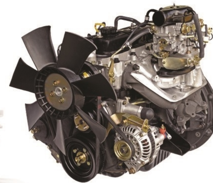
WANFENG 491GP Displacement: 2237 cc Rated output: 41 kW/2800rpm Rated torque: 161 N-m/2000rpm
